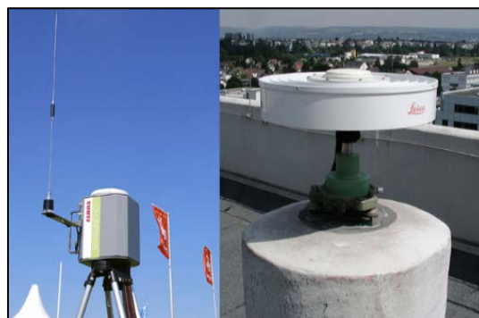
Figure 8. 3: DGPS Reference Stations (With Regular Antenna And Other With A Choke Ring Antenna)
