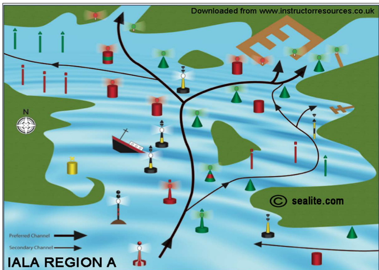
Figure 3. 69: Typical River Channel Marker Buoys (Typical) – Continued
