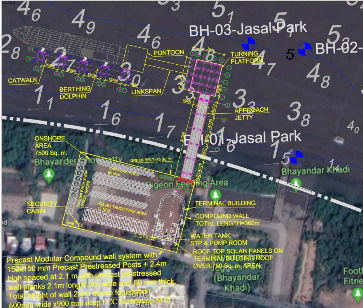
Figure 5. 18: Layout Of Proposed Facilities At Mira-Bhayander Terminal
