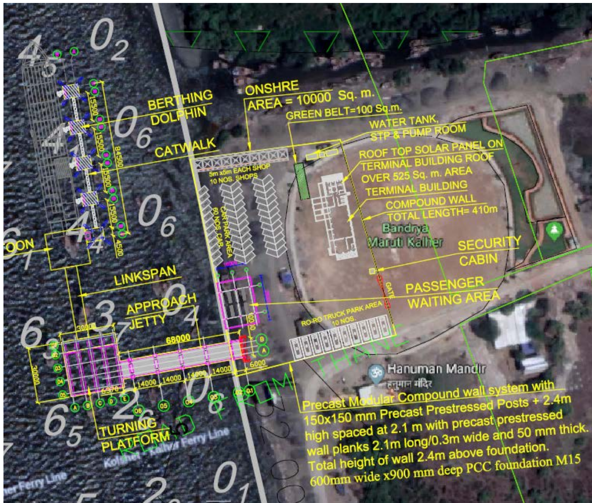
Figure 5. 32:Water Front Facilities At Kalher Terminal
