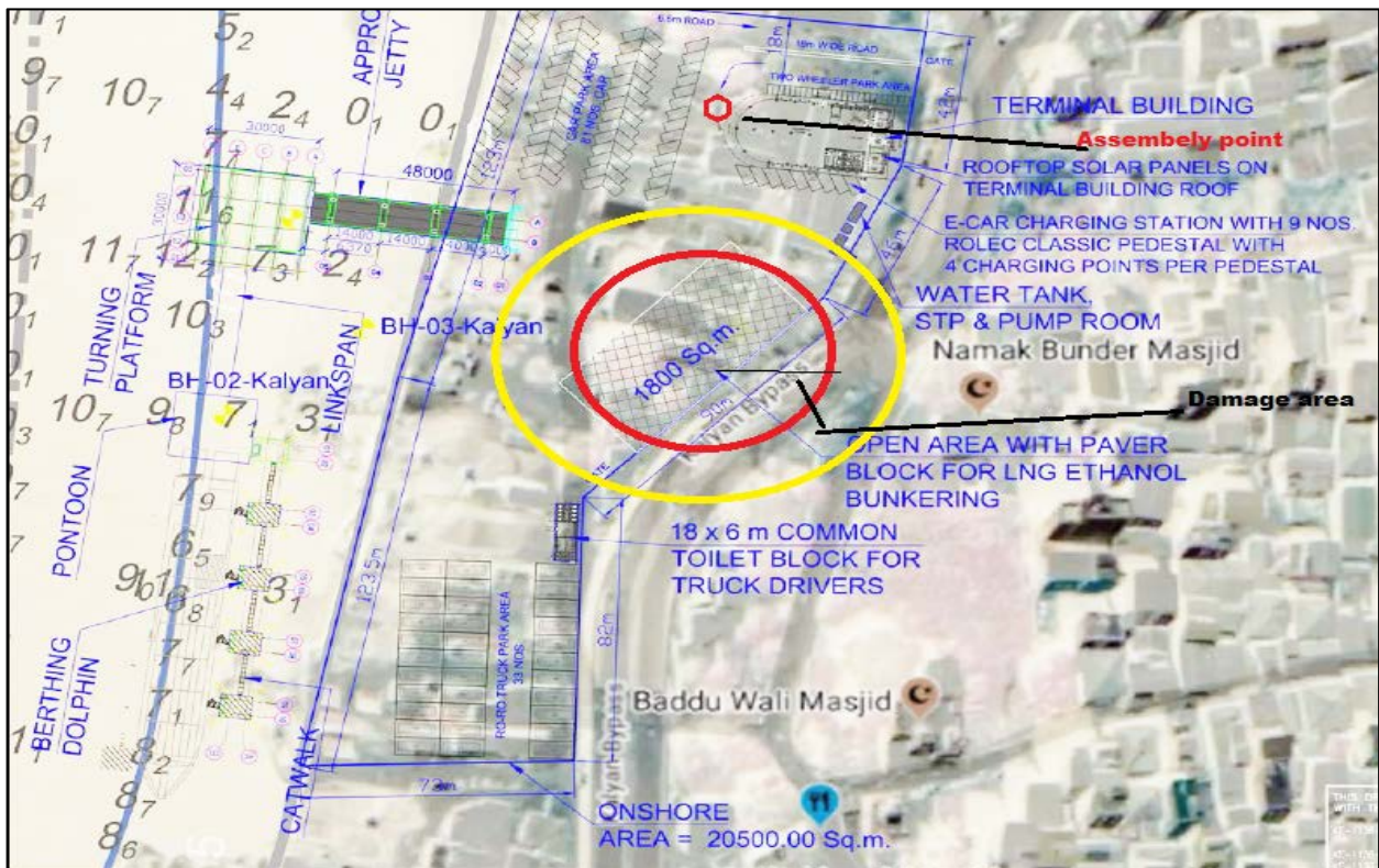
Figure 9. 9: Kalyan Jetty POL Storage Damage Area And Assembly Point During Emergency
