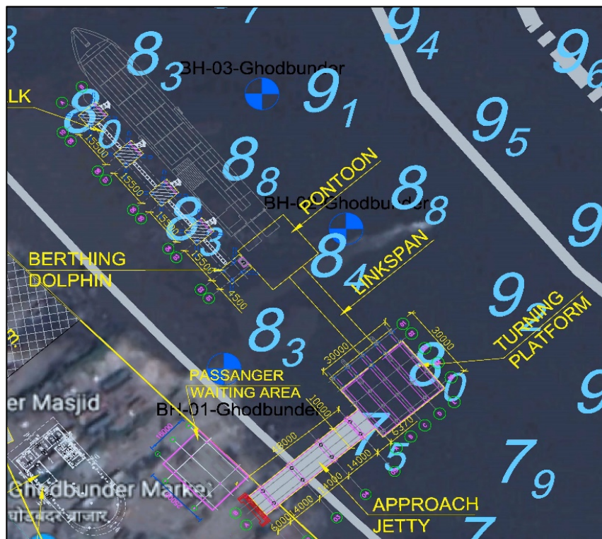
Figure 5. 22: Water Side Layout Of The Proposed At Ghodbunder Terminal On Depth Contours
