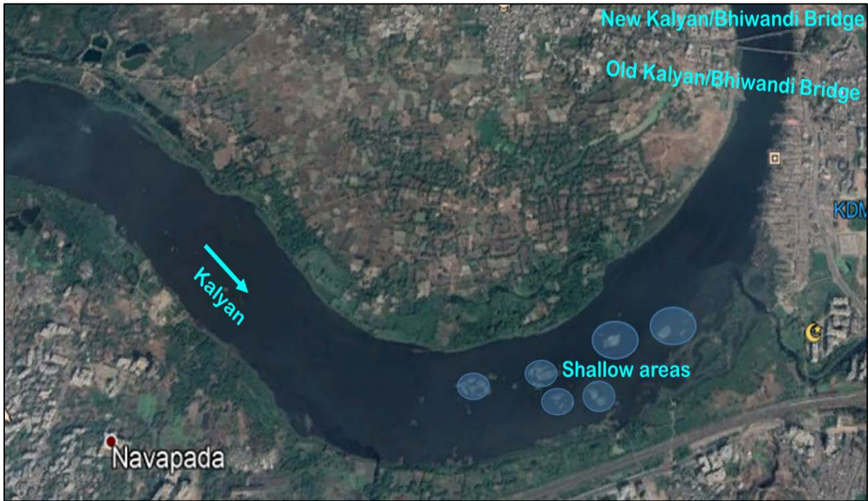
Figure 3. 9: Shoals Staring Around Chainage 47.500 Km To 48.200 Km Showing Shallow Depths
