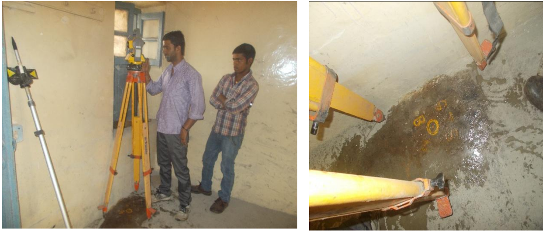
Figure 6 - PWD Benchmark at Kamatagi (ch. 35.37km), referred to GTP-03
