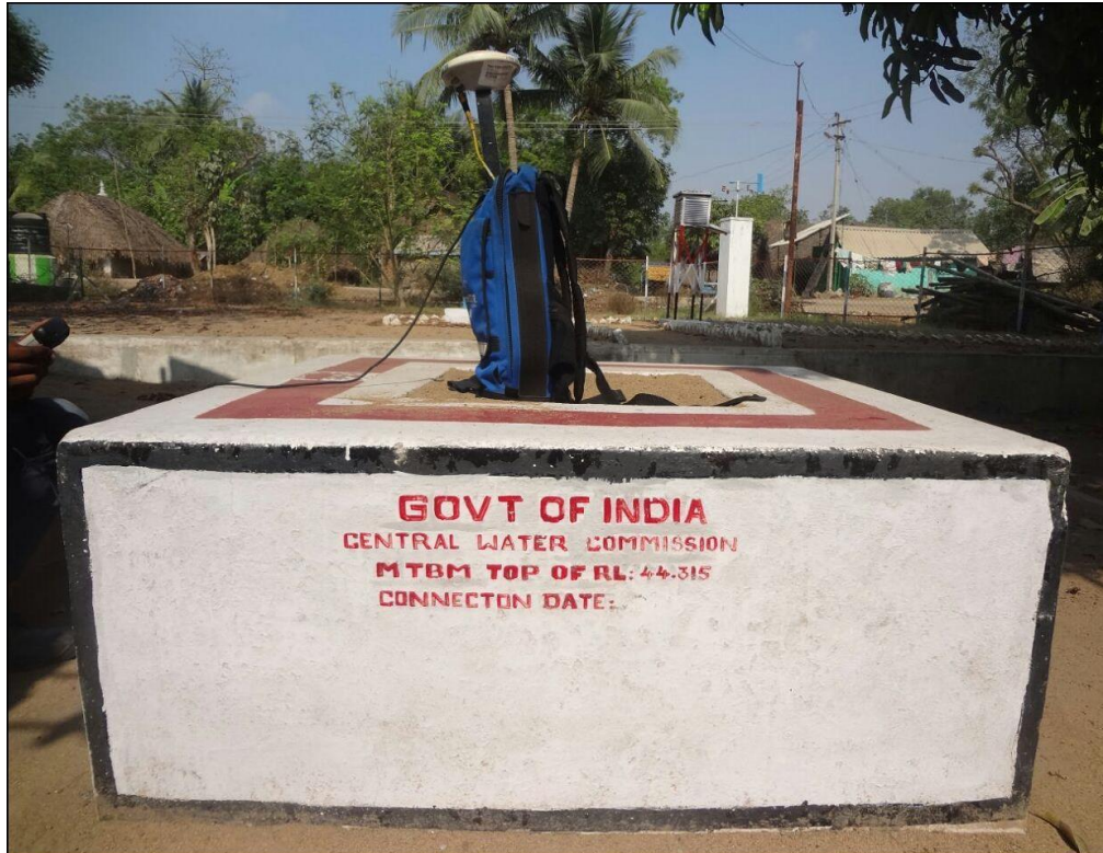
14: MTBM at Villupuram Gauge Station at Chainage 40.9 km
