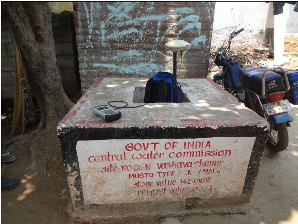
27: Vazhavachanur CWC Benchmark at 103.8 km
