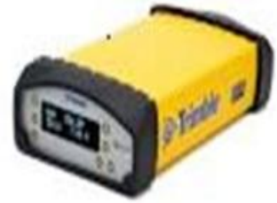
Figure 40- DGPS Survey Instrument
