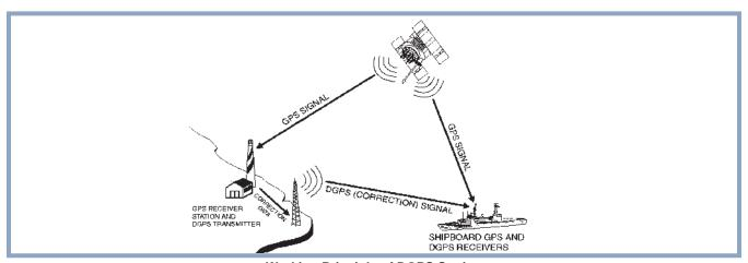
**Working Principle of DGPS Station**
