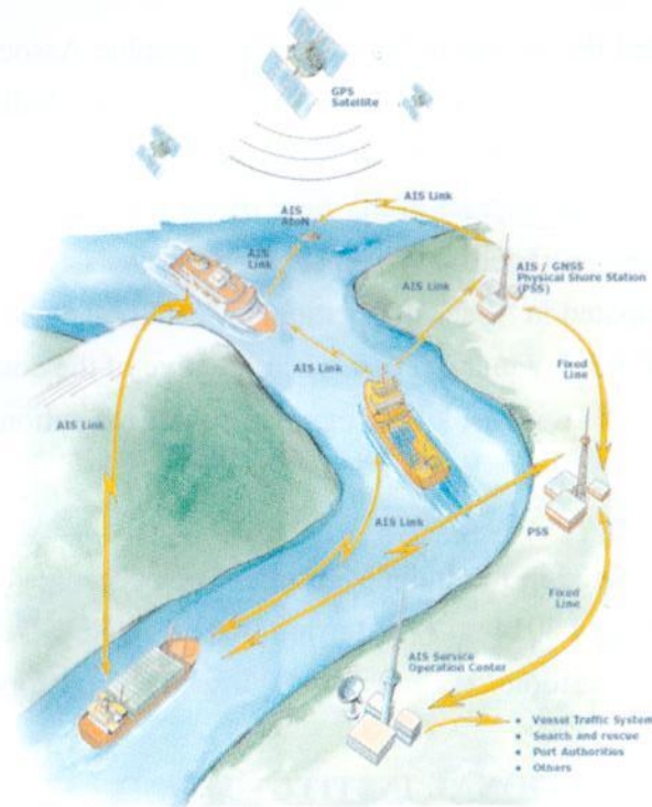
Schematic drawing showing function of River Information system
