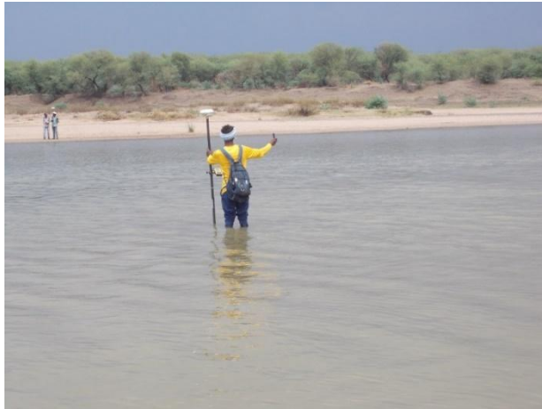
Figure 7 - Spot Leveling by DGPS
