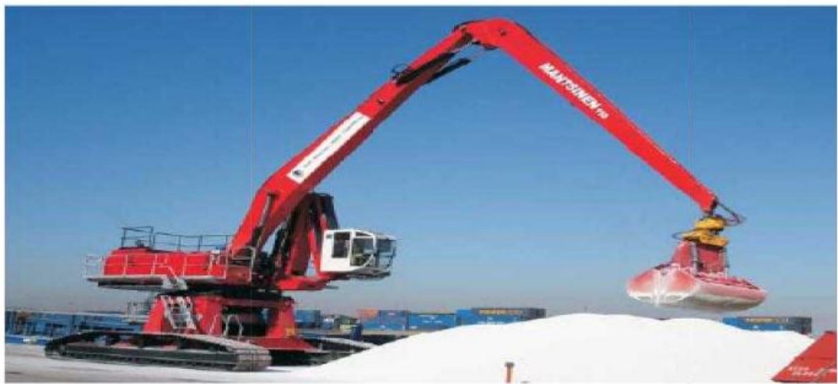
Fig No.5.6 Crawler cranes
