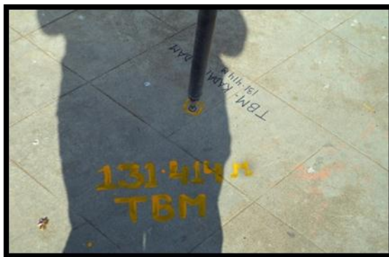
Kadana Dam TBM at Ch 246.9 km
