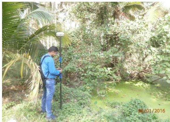
Figure 5- Spot leveling by DGPS in progress
