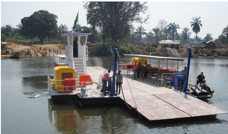
Figure 5.13 A typical modular ferry
