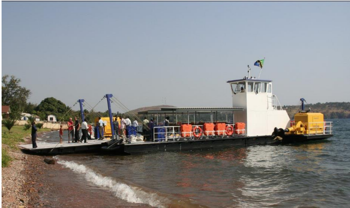
Figure 7.2 A typical modular ferry in operation (note no terminal is needed for loading / unloading)
