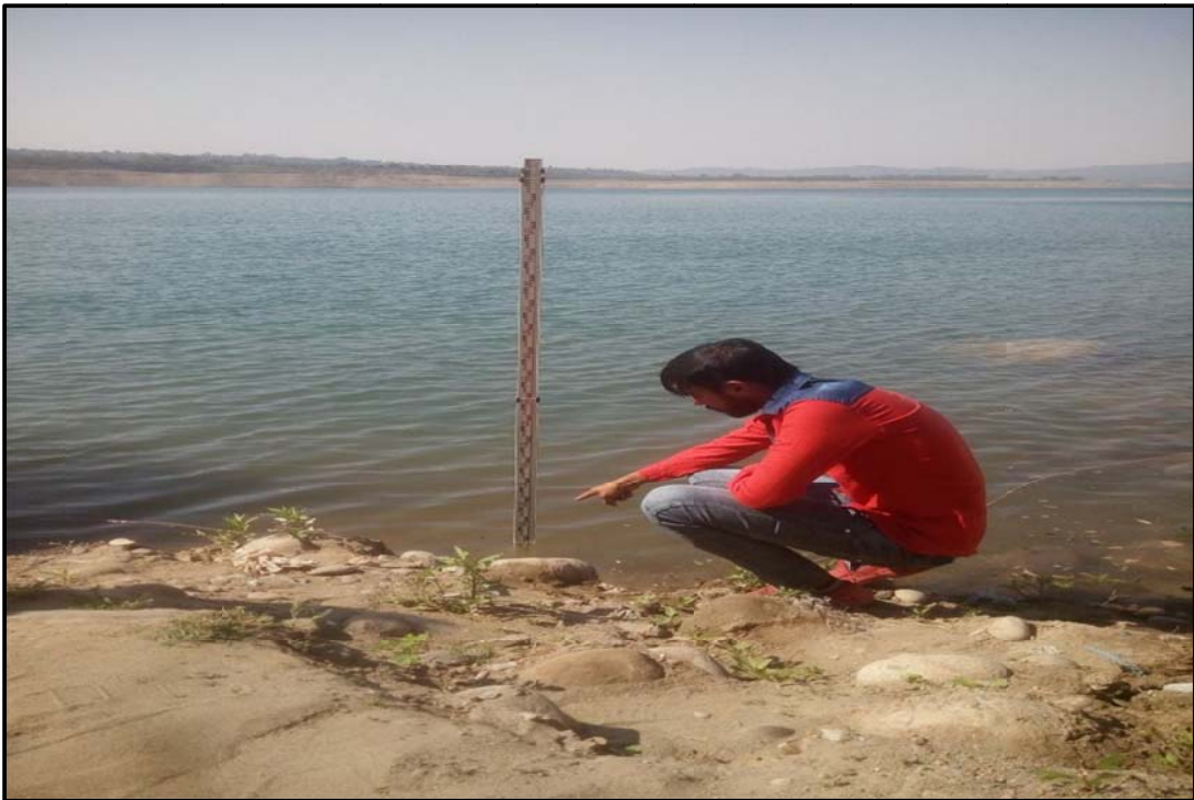
Figure 5 – Ch. 10.00 Km Gauge Fixing During Survey Period
