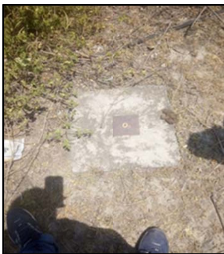
Figure 3 – Bench Mark at Ranjit Sagar Dam used for BM and Control Points
