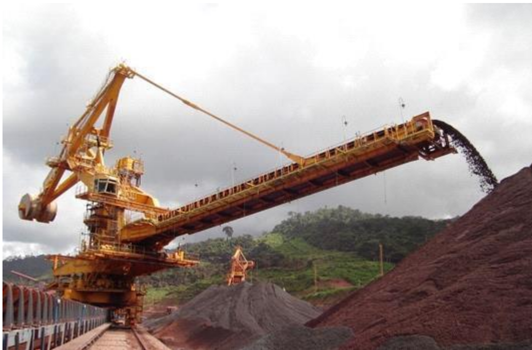
Figure : Typical Arrangement of Stacker
