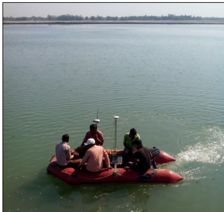
Figure 4- Bathymetry survey work
