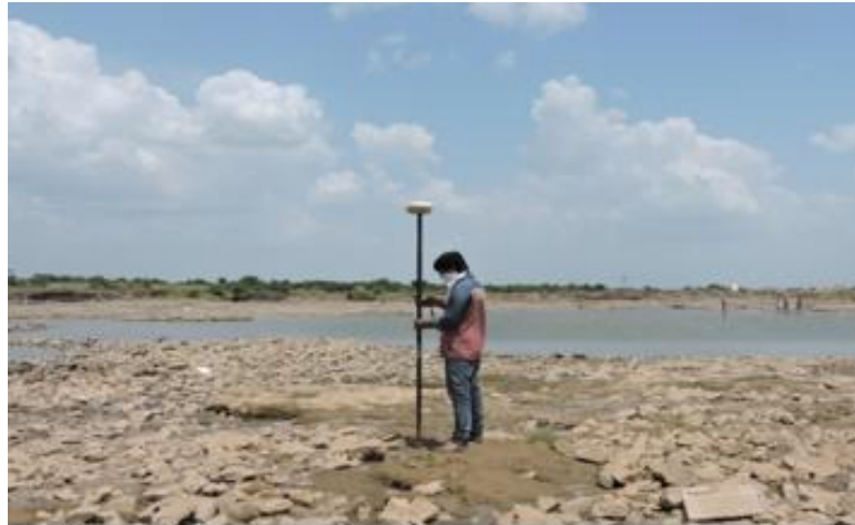
Figure 6 - Spot leveling by DGPS
