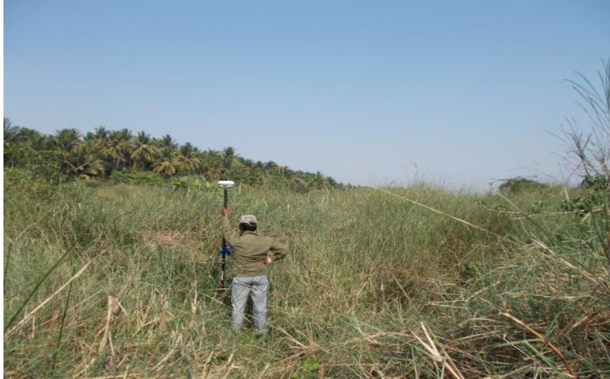
Figure 4 - Spot leveling by DGPS
