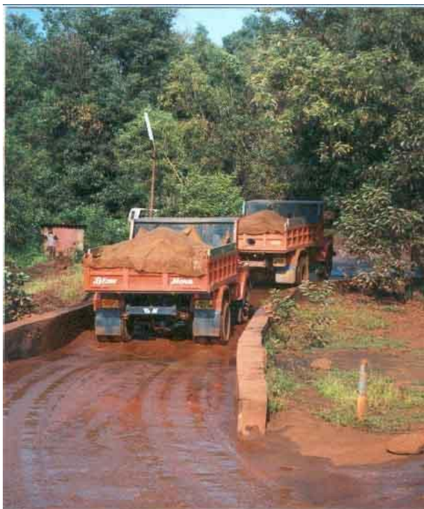
Fig. 5.13: Coverage of the iron ore with tarpaulins
