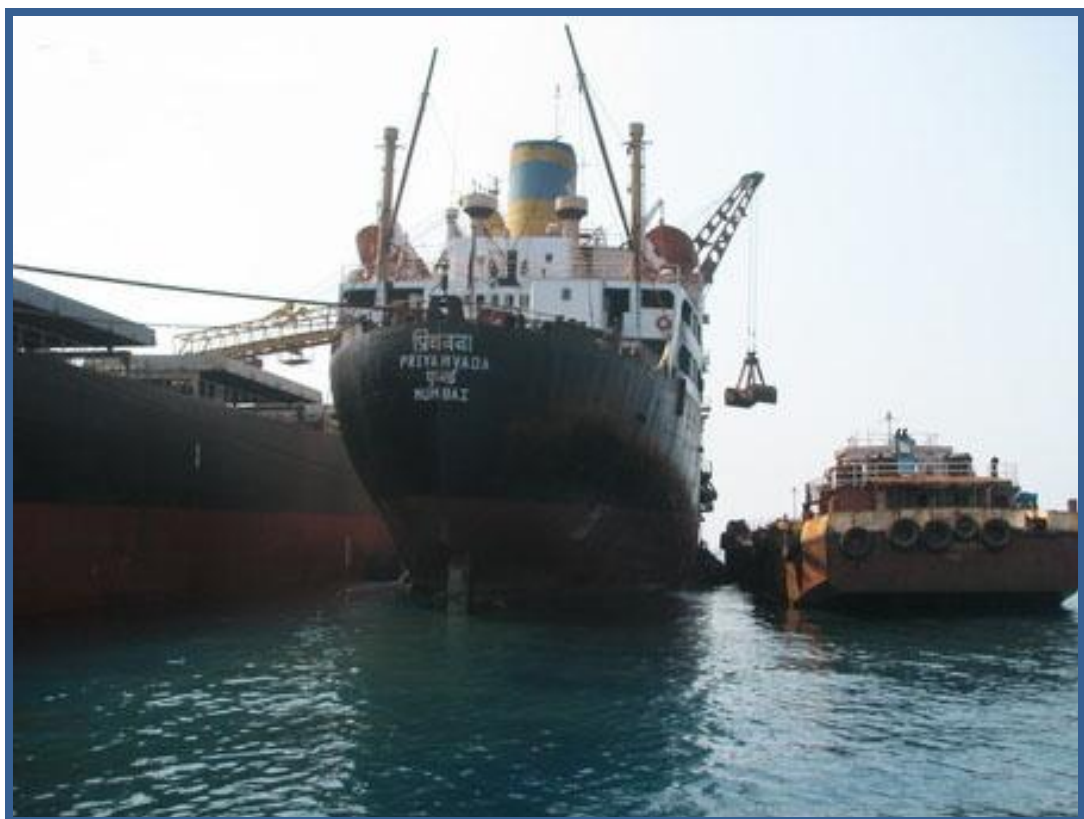
Fig. 3.14: The Transhipper MV Priamvada - loading iron ore in to mother ship anchored mid sea
