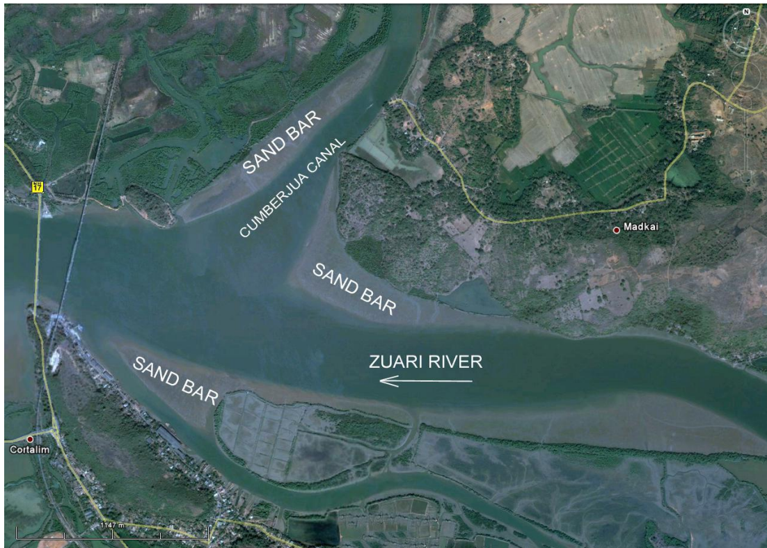
Fig. 4.25: Formation of shoals and sand bars at the mouth of Cumberjua canal with Zuari River
