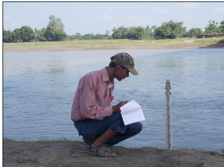
**Figure 46 Tide Gauge Reading**
