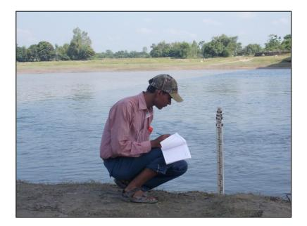
Figure 46 Tide Gauge Reading
