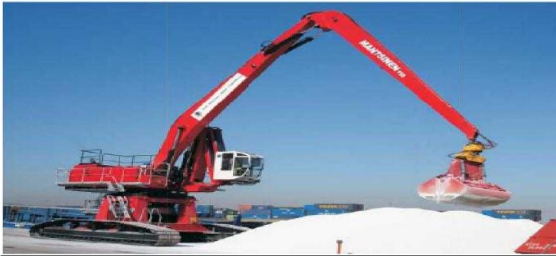
Fig No.5.6 crawler cranes
