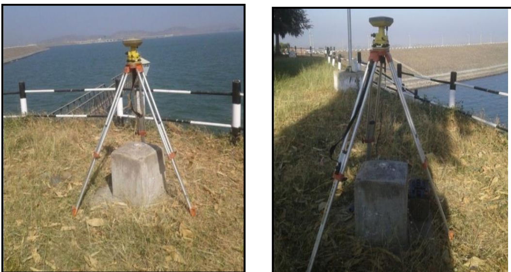
Figure 2.1 – Bench Mark (GTS BM-1) at Upstream of Ukai Dam used for Control point
