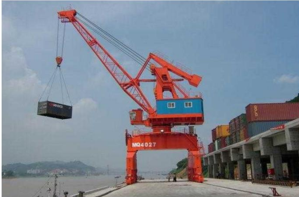
Fig No.5.3 Level Luffing Crane
