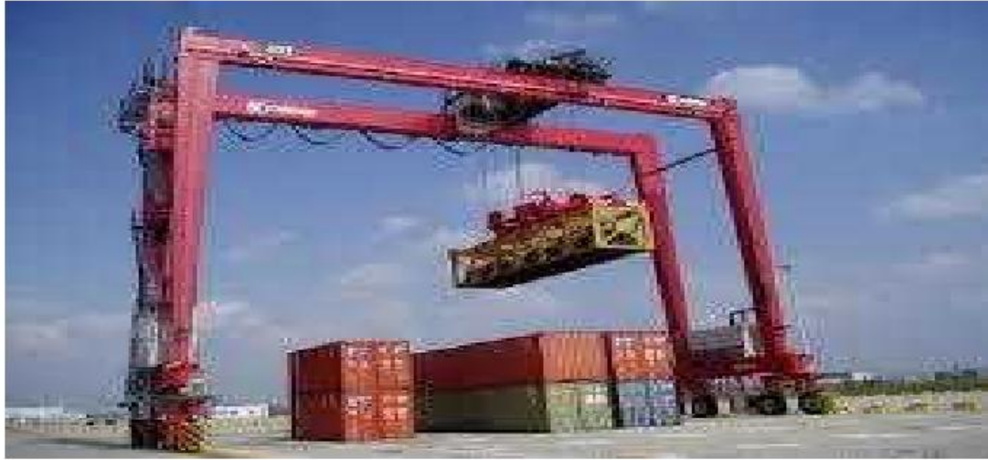
Fig No. 5.2 Rubber Tyre Gantry Crane
