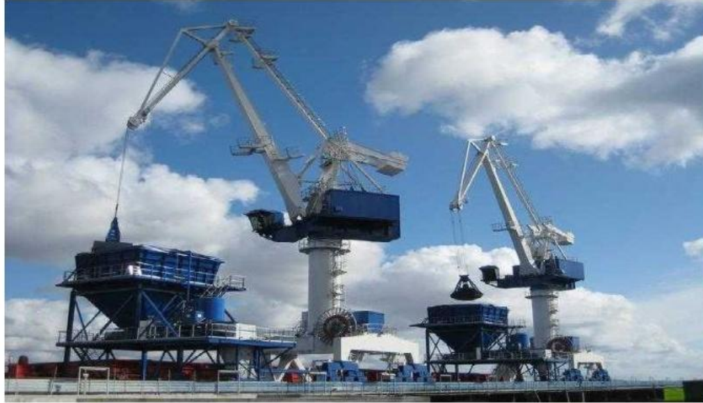
Fig No. 5.4 Grab Type Level Luffing Crane
