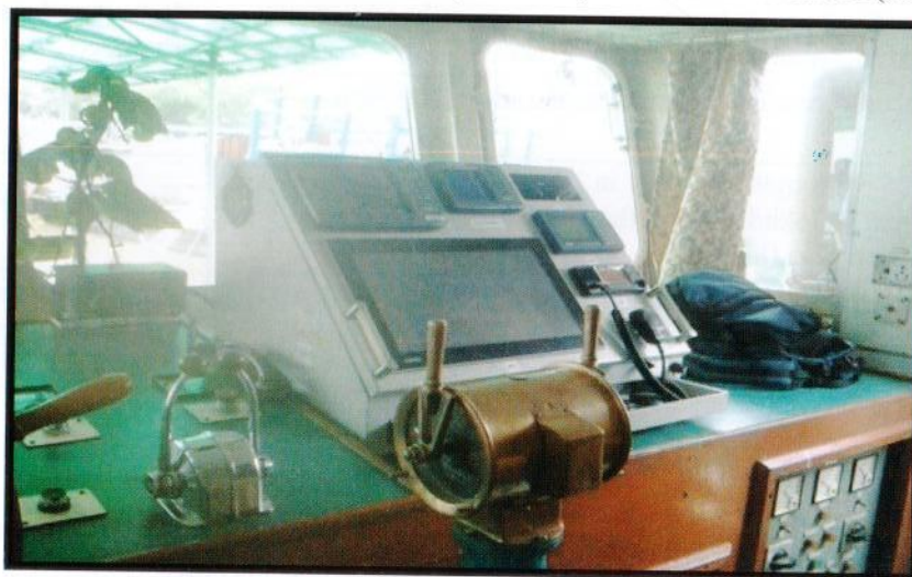
RIS equipment onboard IWAI vessels
