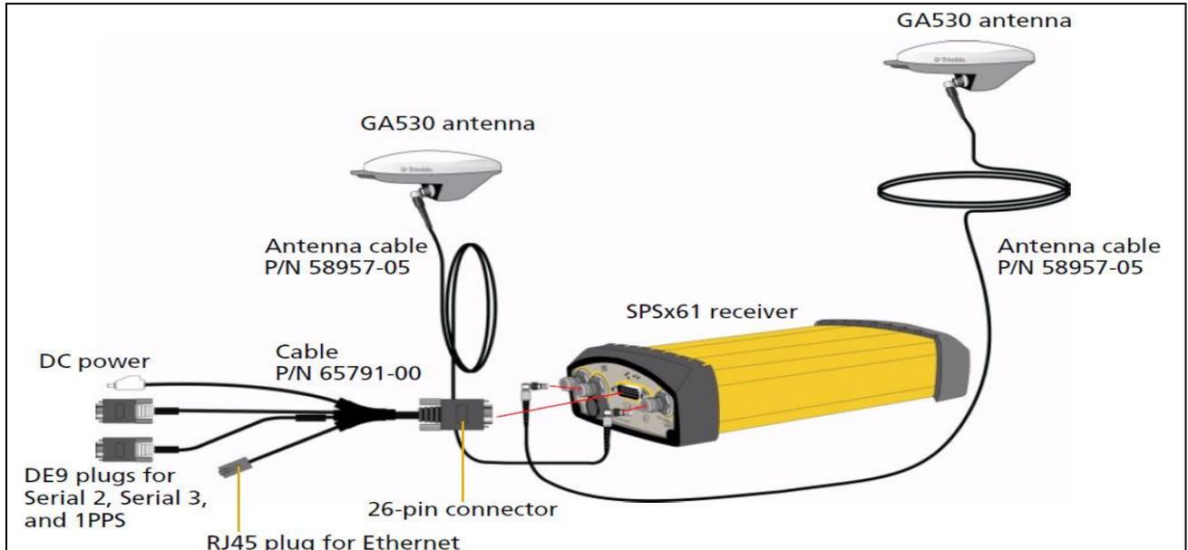
**Figure 3.4: Equipment Diagram**
