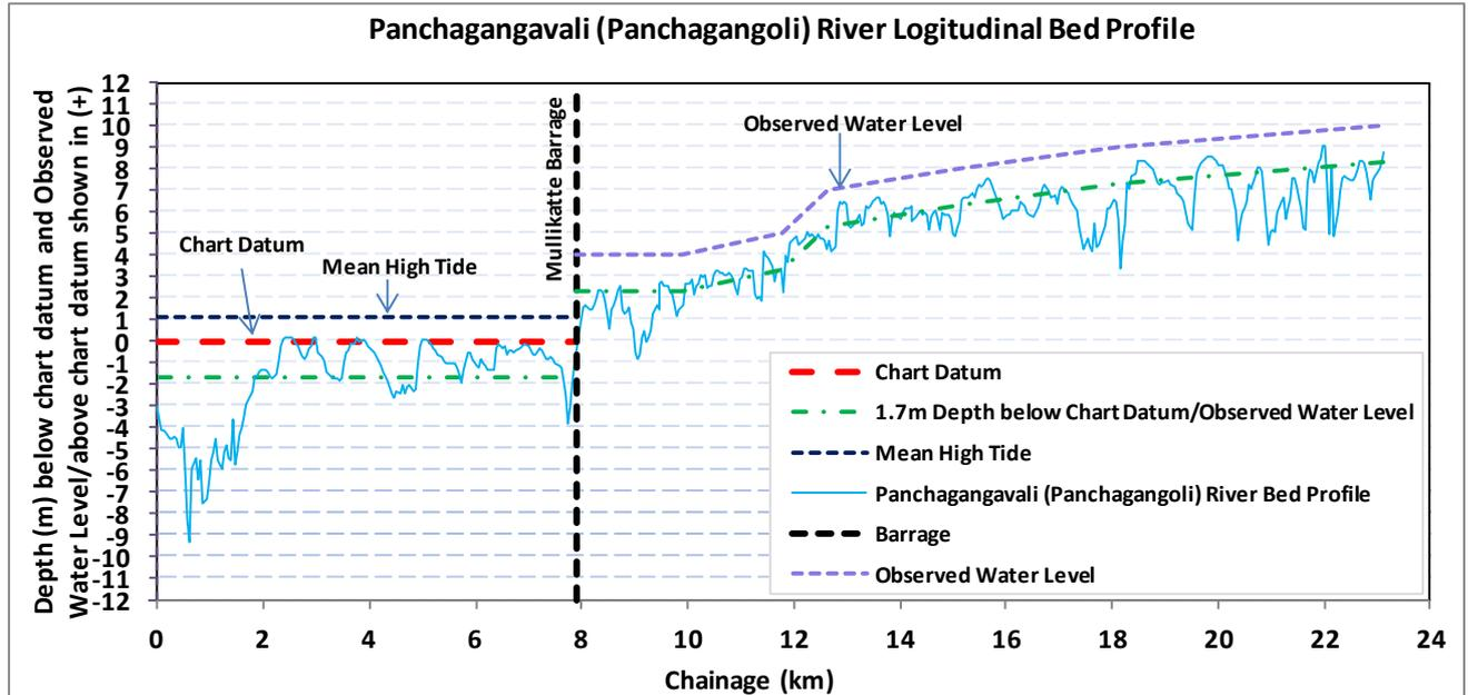
**Figure 3.13: Longitudinal River Bed Depth Profile of Panchagangavali (Panchagangoli) River from Ch 0.00km to Ch 23.13km**
