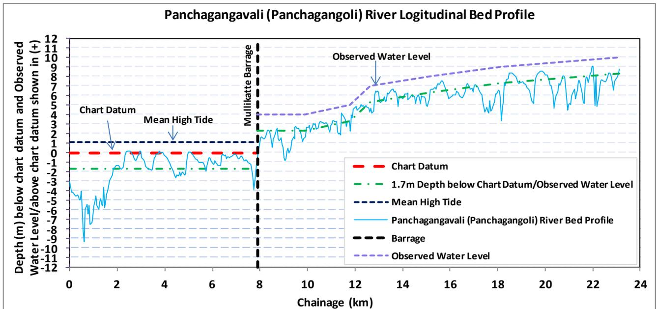
5. Feasibility study suggests that the river is safely navigable between chainage 0.00km - 7.82km and chainage 7.90km – 23.13km. Mullikatte Barrage exists at 7.82km – 7.90km.
