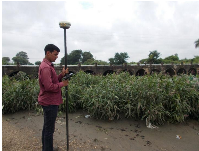
Figure 3 - Spot leveling by DGPS
