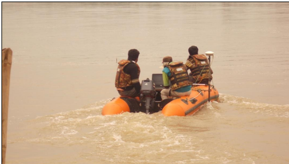
Figure 4- Bathymetry survey work
