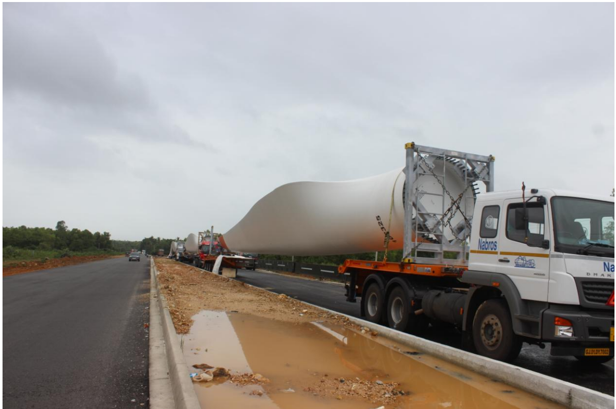
Figure 4.2: Wind Turbine Blades Transported via Trailers
