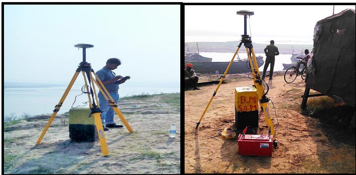
Static Observation at Ch. 5.40 km & Ch. 59.00 km
