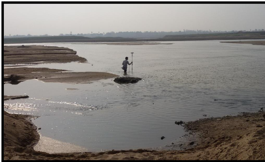
Topographic Spot Levelling by Trimble DGPS
