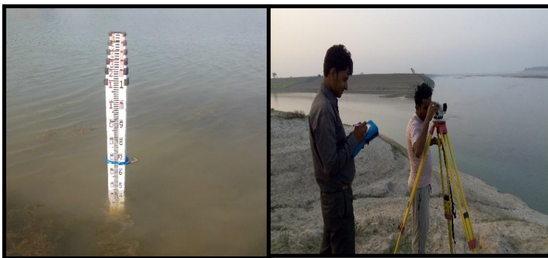
Levelling & Tide Observation at Pillar No 01 Ch. 0.100 km
