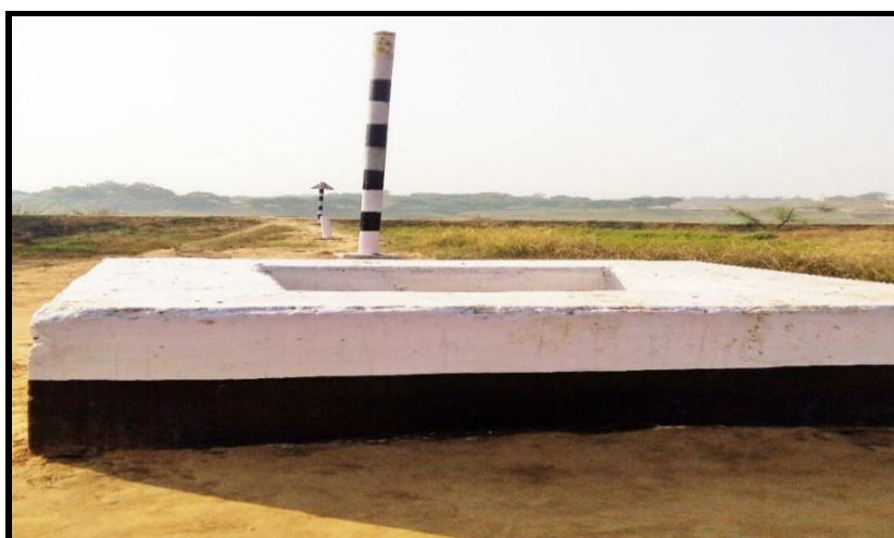
CWC BM at Meja road, Allahabad at Ch. 10.21 km
