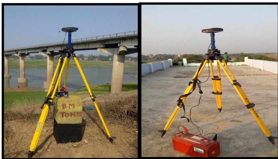
Static Observation at Ch. 9.82 km & Static observation at Meja Road Base
