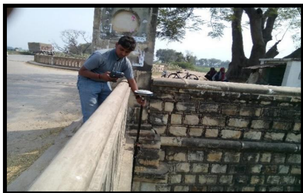
Topographic Spot Levelling by Trimble DGPS
