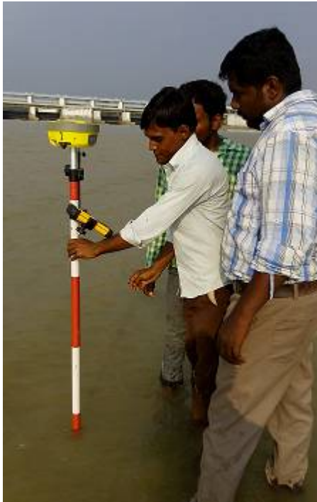
Figure 4- Spot leveling by DGPS
