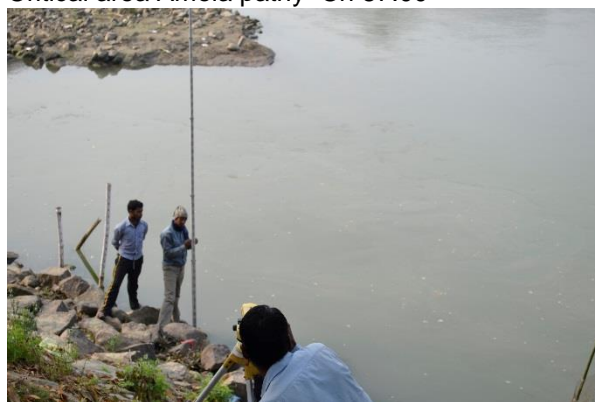
Shifting the RL in the water
