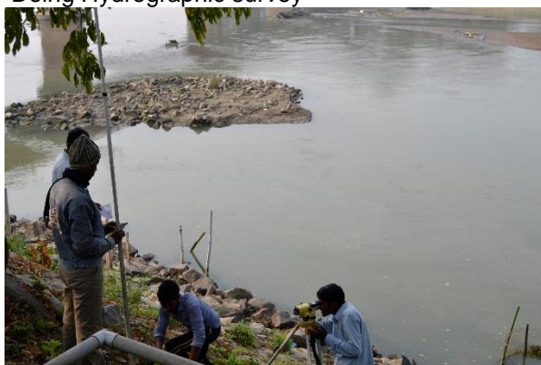
Transferring RL Through Auto level
