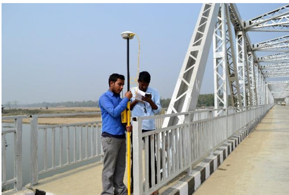
Figure 14 Topographic survey using South RTK instrument near Dhansari Bridge no-2 (Ch. 33.17 km)
