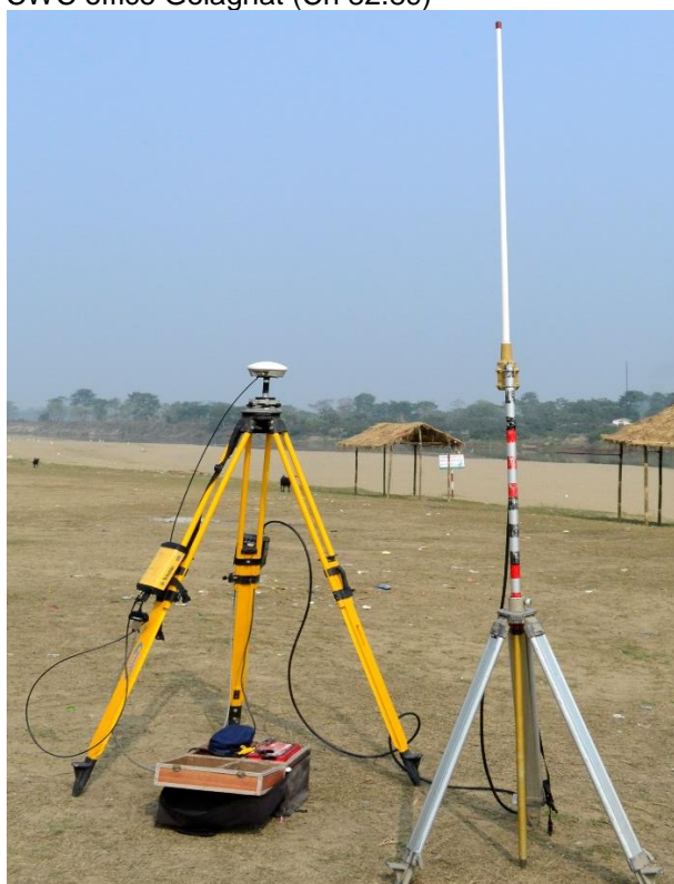
TRIMBLE RTK-Base Station
