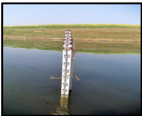
Tidal Observation at Ch.8.64 km
