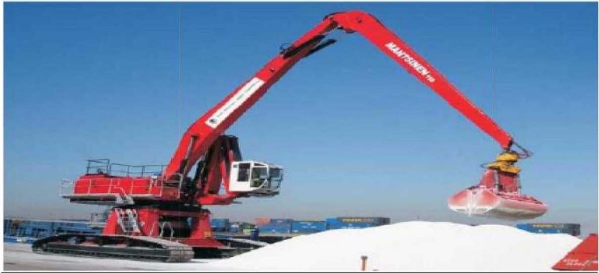
Fig No.5.6 Crawler cranes
