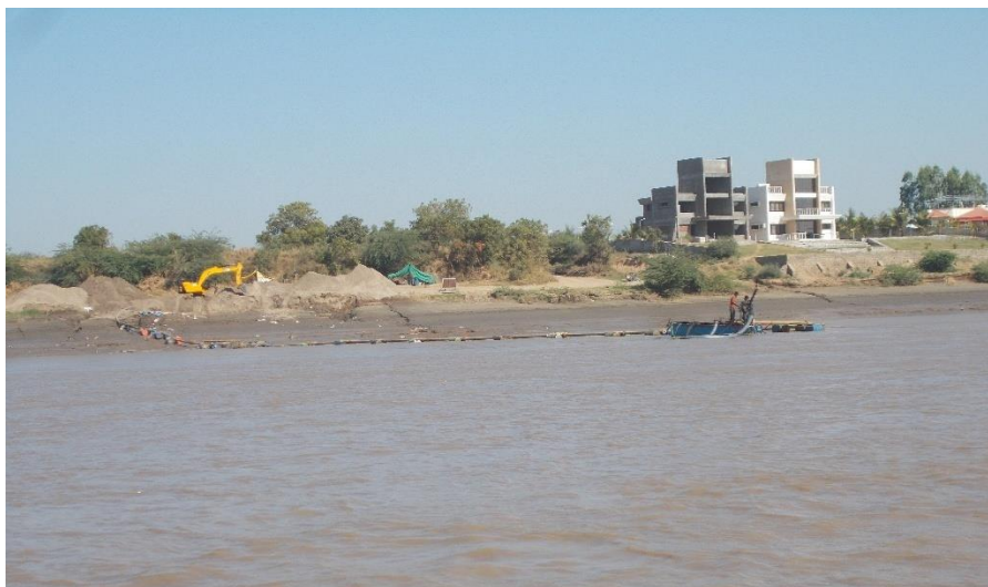
Figure 2.10 – Mining of Sand using Suction Pump
