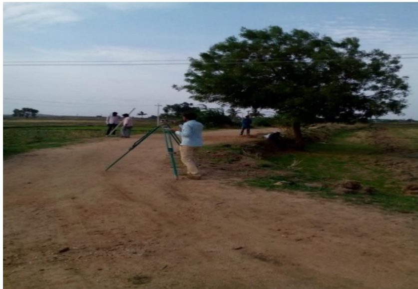
Figure 4 - DGPS Spot Leveling Comparison by Auto Level
