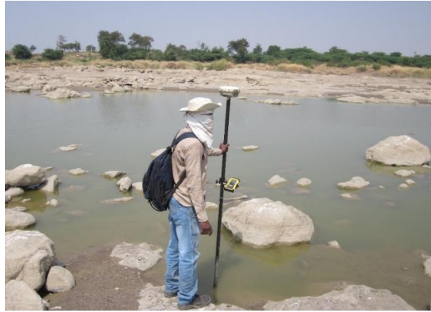
Figure 4 - Spot leveling by DGPS
