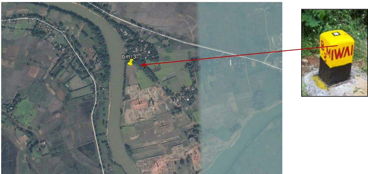
Figure 25-Bench Mark Form & Google image view of BM-3
