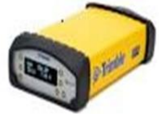
Figure 19- DGPS Survey Instrument
