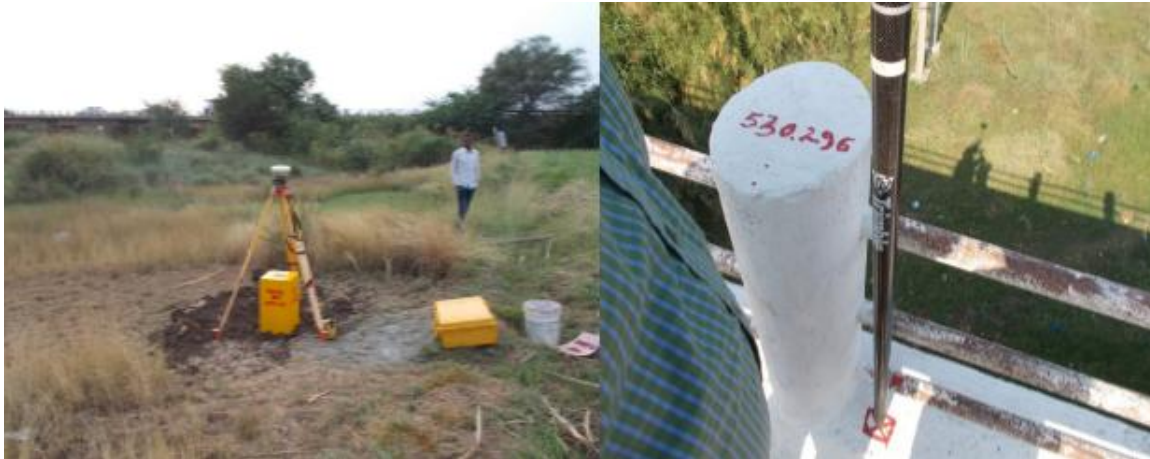
Figure 6 - PWD Benchmark upon Chinchakhandi Bridge, referred to GTP-03
