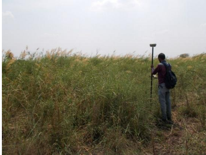
Figure 5 - Spot leveling by DGPS
