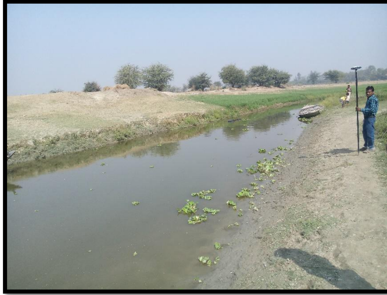
Topographic Spot Levelling by Trimble DGPS
