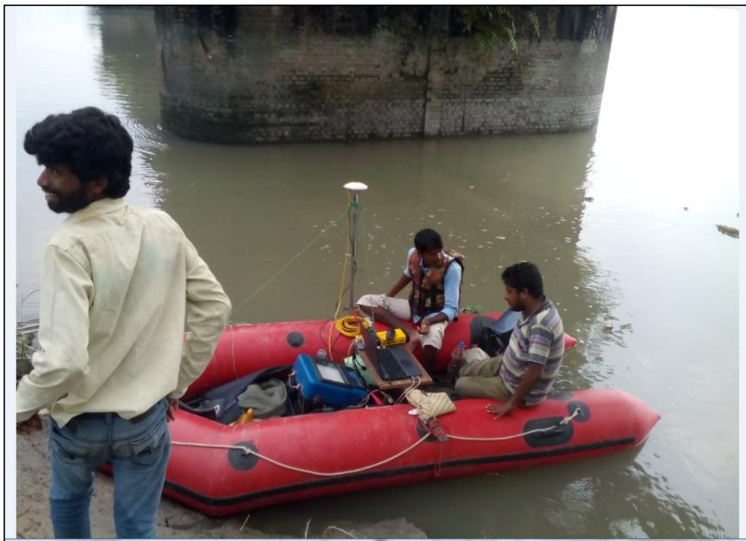
Figure 25- B.M pillar Establishment & Bathymetry Survey Instrument
