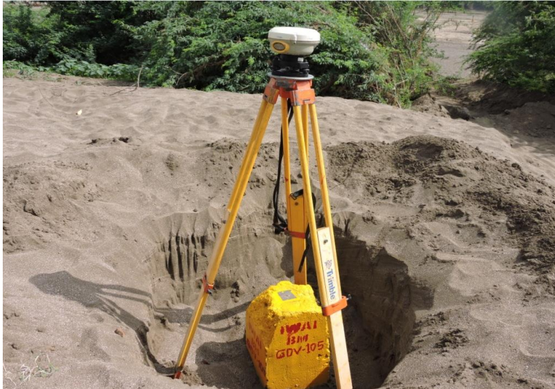
Figure 9 - Sand deposition over BM pillar
