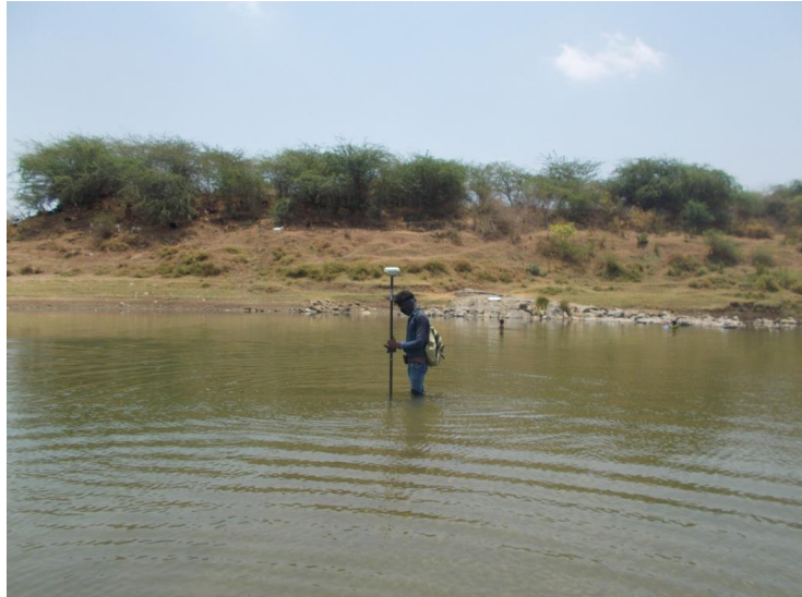
Figure 6 - Spot leveling by DGPS
