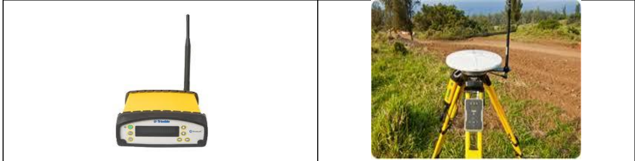
Figure 12: Topographic Survey Instrument (Two Trimble SPS 855 RTK System)
