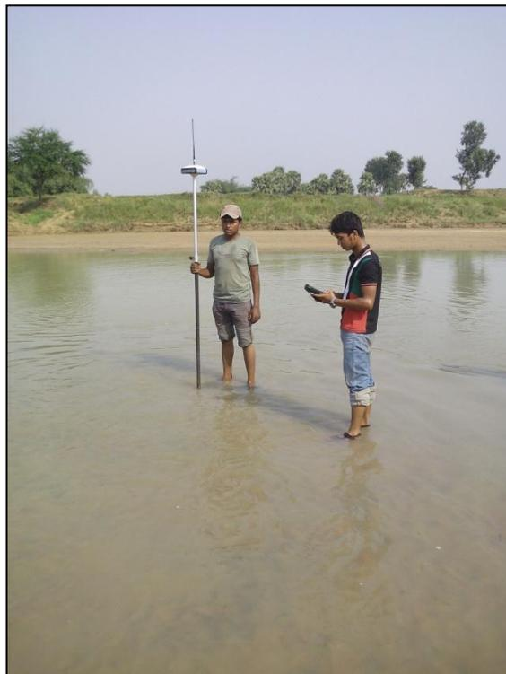
**Figure 53- Topography survey Instruments**
