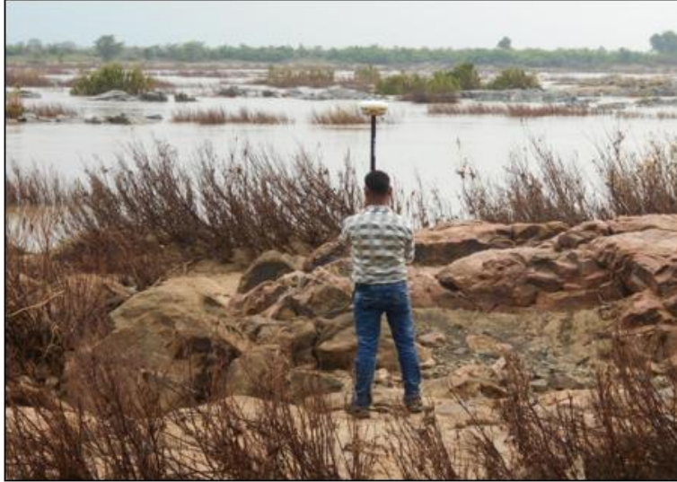
Figure 5 - Spot levelling by DGPS
