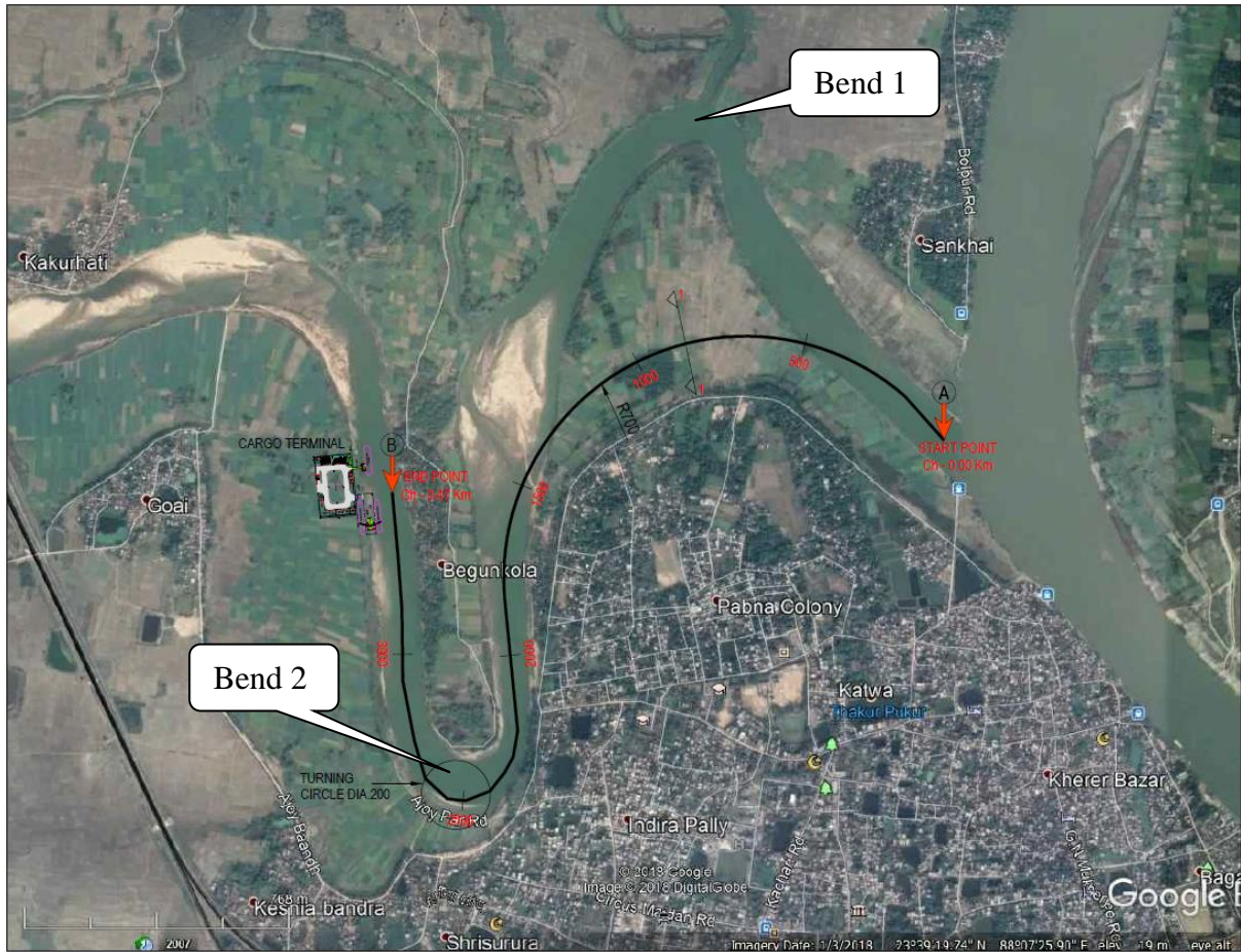
Figure 19: Layout plan of proposed fairway stretch for Ajoy Waterway
