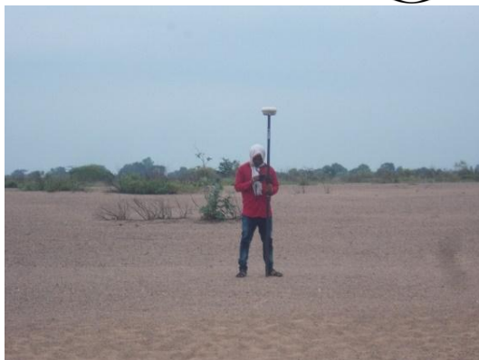
Figure 4 - DGPS Spot Levelling in Progress
