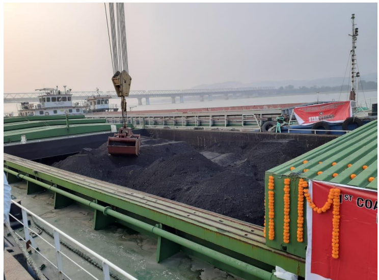
Figure 24- NW-2: Coal handling operations at Pandu terminal
