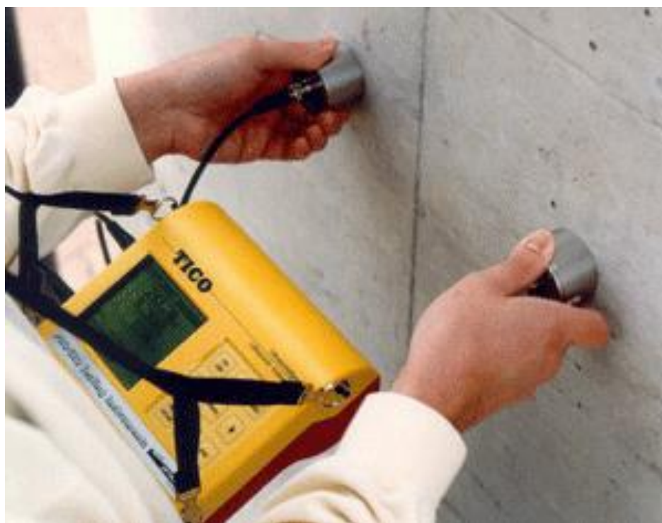
Figure 3: Sample image of conducting UPV tests above water
