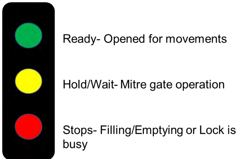
Figure 8.6 Schematic diagram of separate signal system of navigation lock
