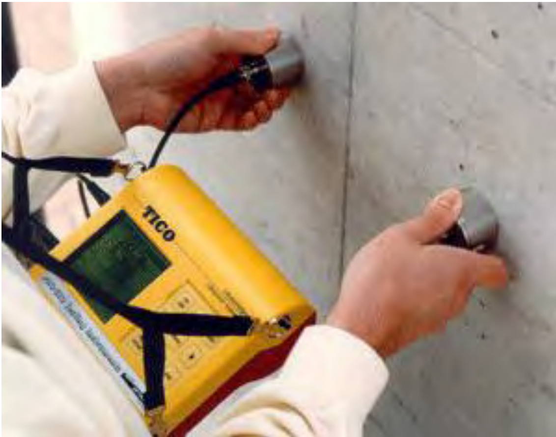
Figure 4.1 Sample image of conducting UPV tests above water
