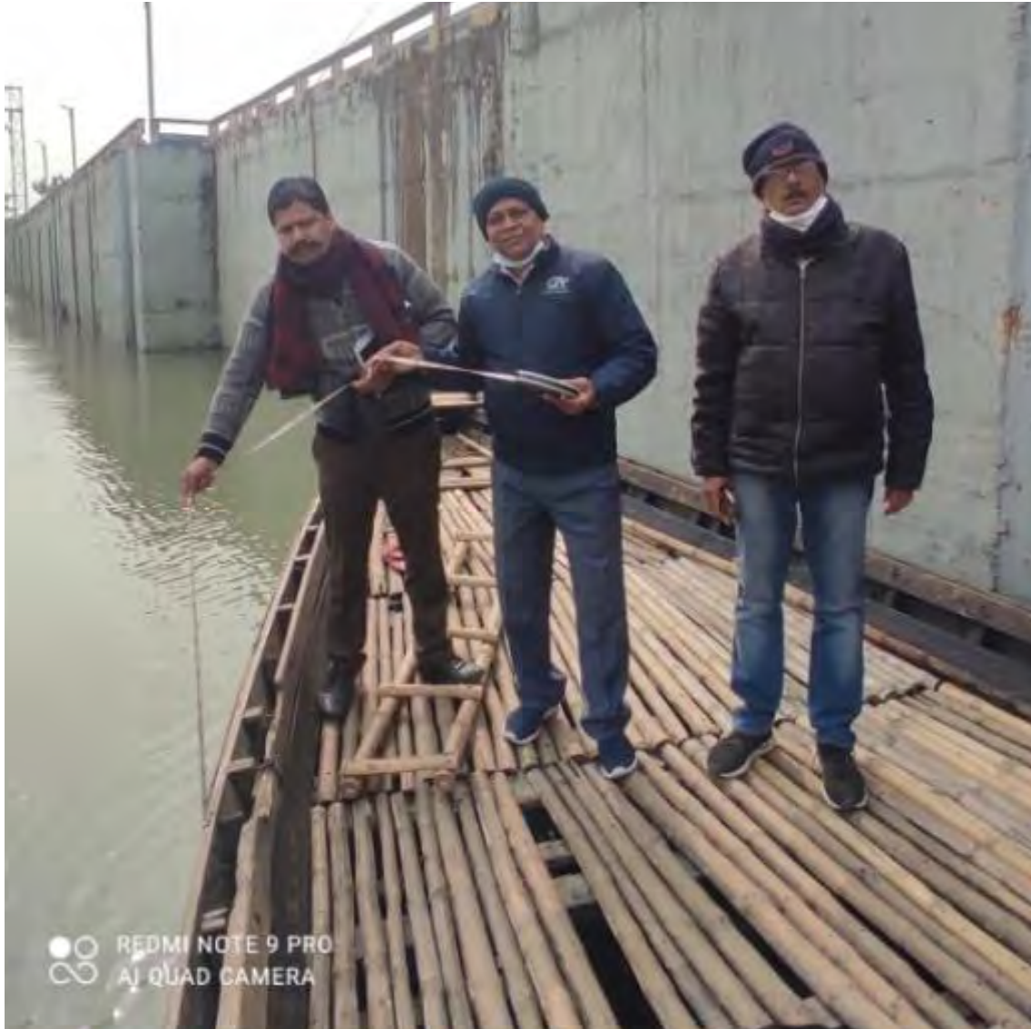
Figure 5.4 Depth measurement in lock chamber for silt deposition over base slab
