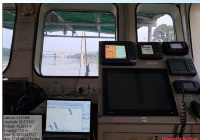
Thalweg Survey in National Waterways using Survey Vessel
