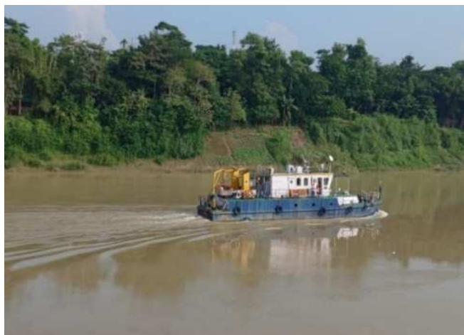
Thalweg Survey in National Waterways using Survey Vessel
