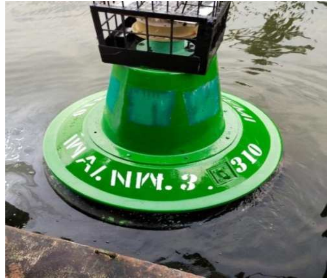
Solar light fitted FRP Buoys
