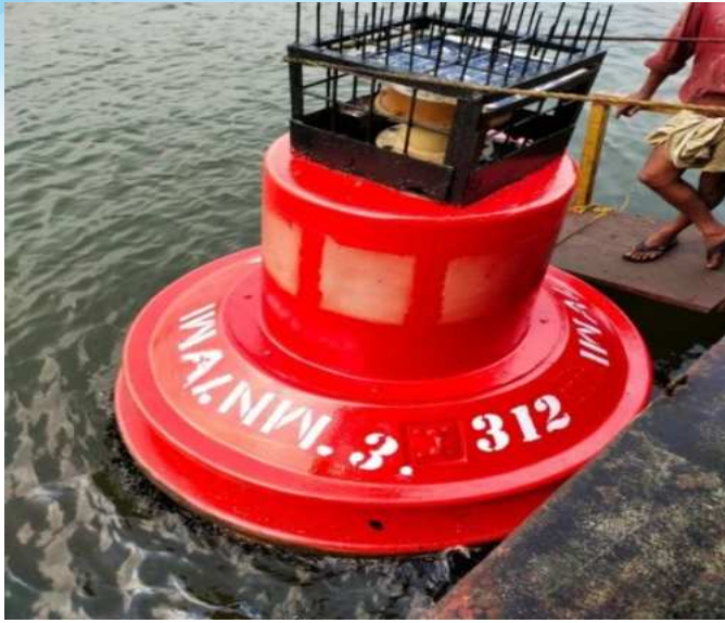
Solar light fitted FRP Buoys
