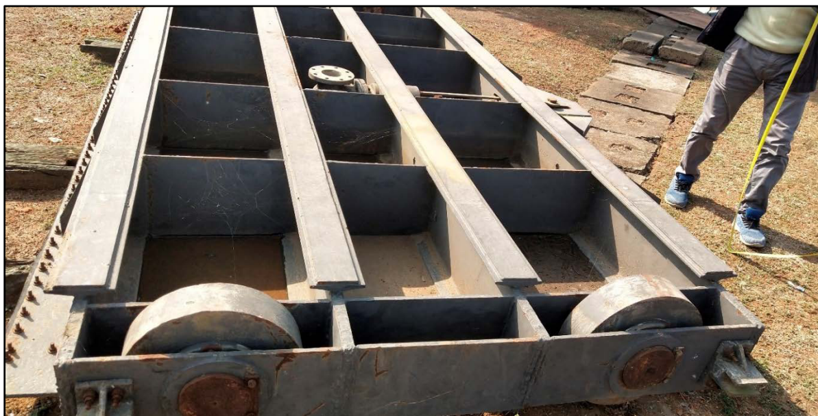
Figure 4.11 Bulkhead Gates for Radial Gate Maintenance
