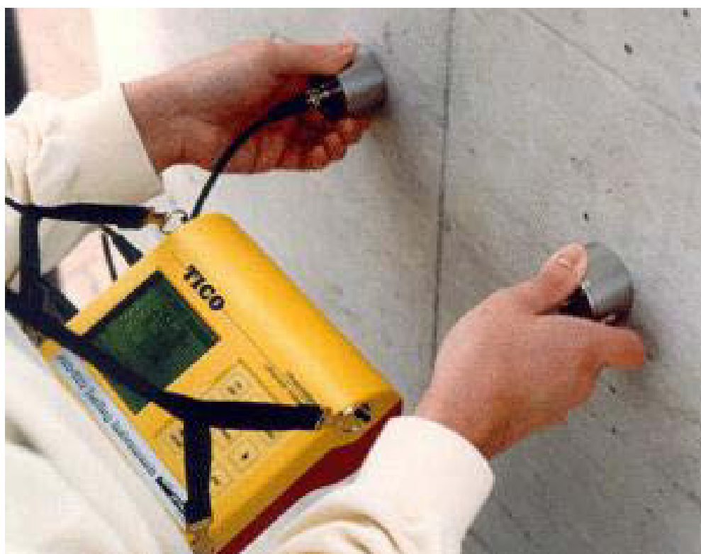
Figure 6.3 Sample image of conducting UPV tests above water
