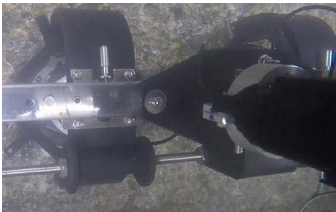
Figure 6.6 Planys ROV integrated with indigenous UPV payload conducting underwater UPV tests.
