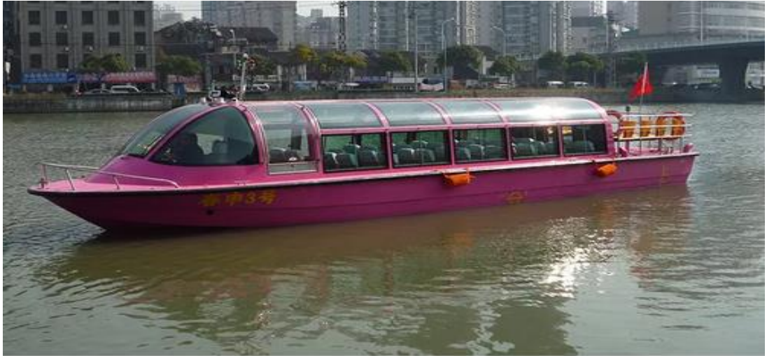
Figure 7-2: FRP Water Taxi Without Engine – 40 Pax
