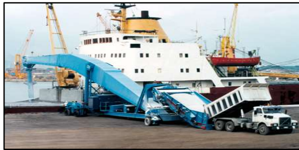
Figure 5.10: A dumper unloading dry bulk cargo and dumper loaded at the berth
