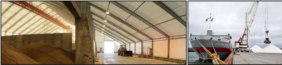
Figure 5.2: A typical dry bulk warehouse and a grab crane unloading dry bulk
